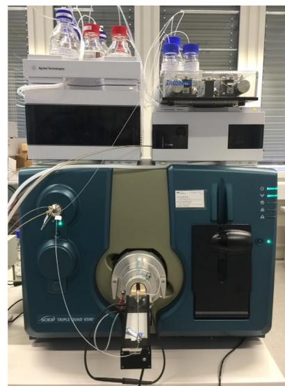
Figure 3: HPLC-MS/MS system with micro-flow setup
