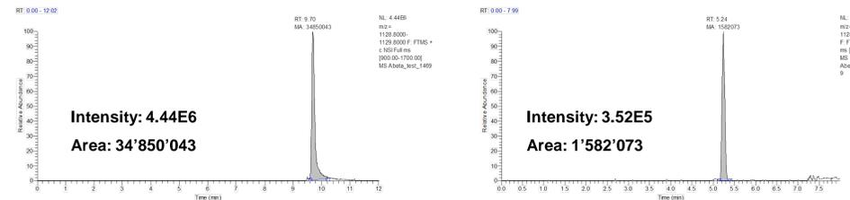
Figure 3: Extracted ion chromatogram of A $\beta$  1-42 of a standard sample, micro-flow set-up (left), regular flow set-up (right)
