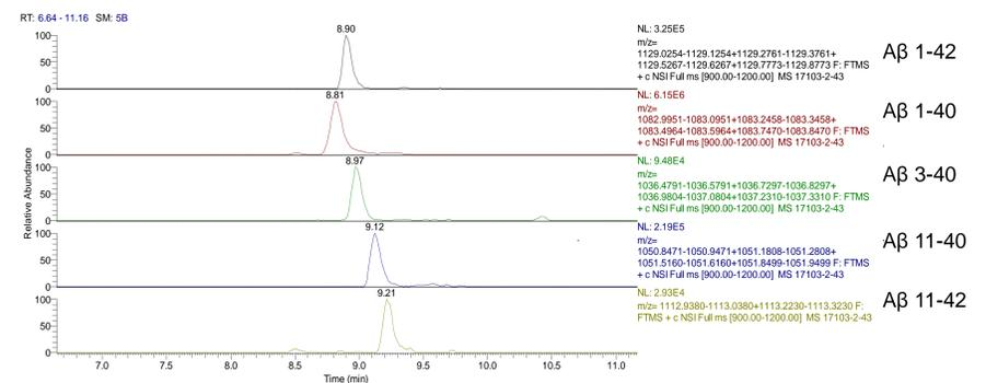
Figure 4: Extracted ion chromatograms of QC substrates detected in human CSF
